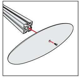
**Base Plate & Extrusion Connection**
