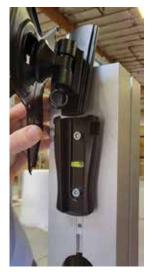
Slide V4 Connectors into groove of Extrusion. Tighten Set Screws to secure connectors in place.
