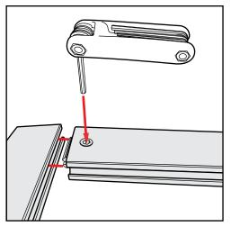
**Extrusion & Lock Connection**
